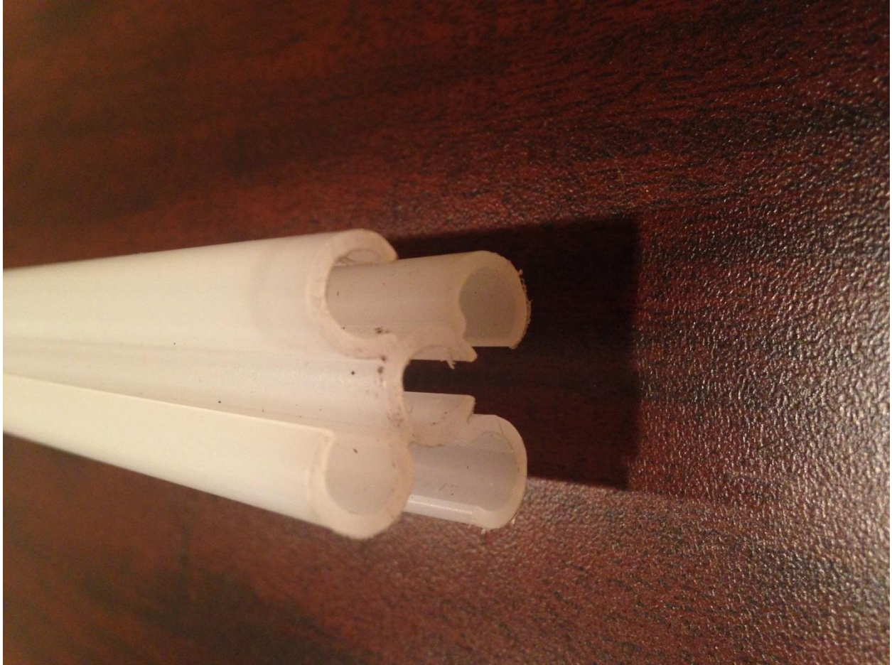
Figure 1. EGRP ® tube extrusion showing crescent-shaped elements clustered together.
